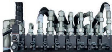
HYDRAULIC CONTROL BOOM PROPORTIONAL DIRECTIONAL SPOOL VALVE
