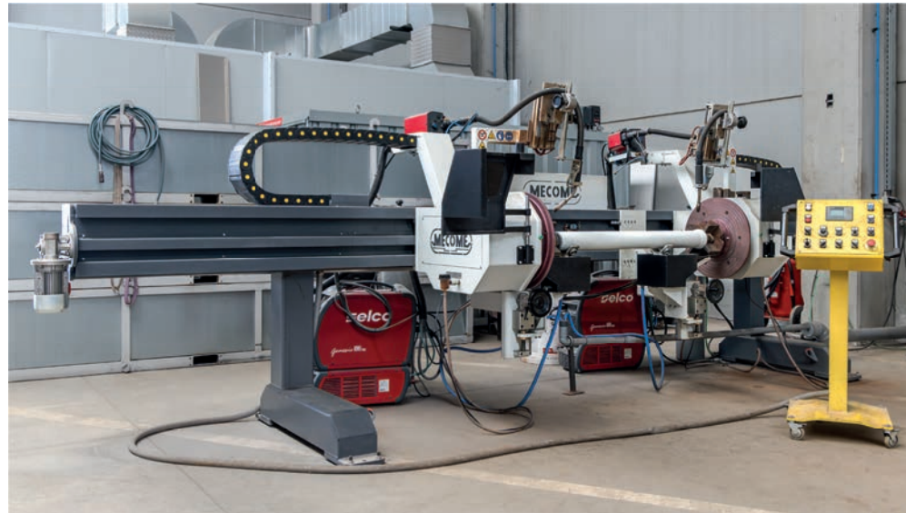
Automatic welding robot with cooling for welding of single- and double-walled concrete pipelines
