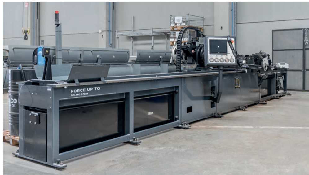
Test - disassembly and assembly bench for all types hydraulic cylinders
