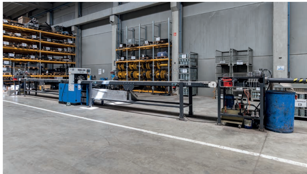
Hose press for manufacturing of customised concrete hose
